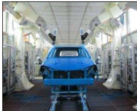
Water Borne Paint & 3 Wet Painting Technology (VOC reduction - 50%)
